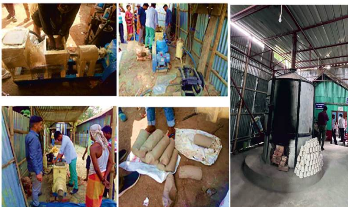
Fig. Installation and operation of de-airing pugmill and wood fired kiln at Asharikandi Cluster
