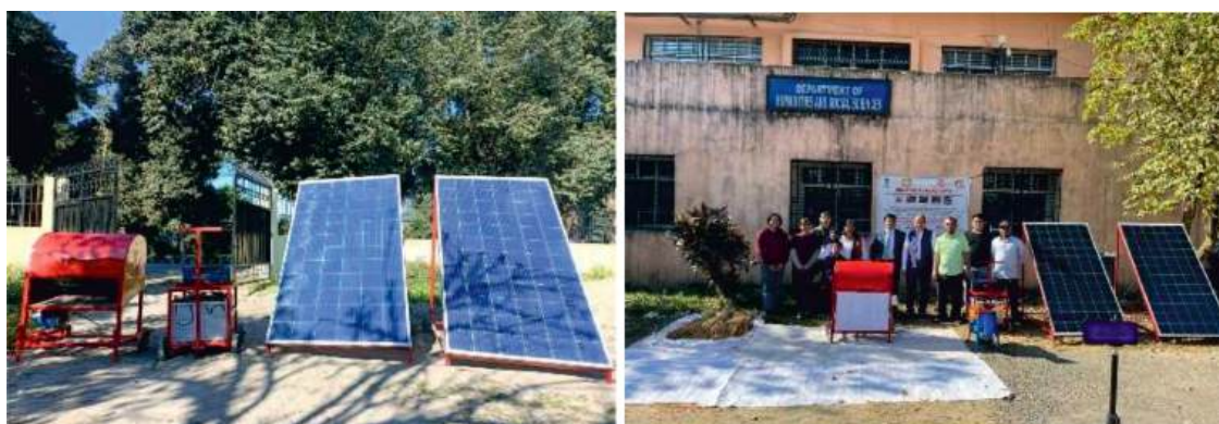
Fig.: Solar powered paddy thresher developed by Dept of Agricultural Engineering, NERIST
